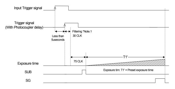
Note 1: The trigger signal will be removed by the filtering if the pulse width of the input trigger signal is less than 30 CLK. Please input a trigger signal with more than 31 CLK pulse width.
